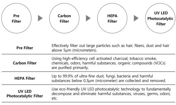
% Carbon Filter and HEPA Filter are integrated Filters.
