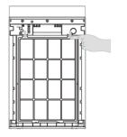
To access the prefilter, remove the front cover from the device.
