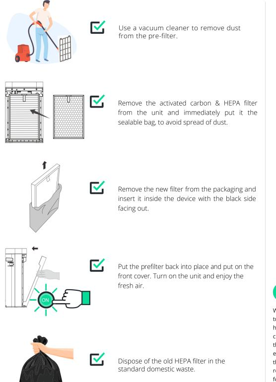
We recommend to turn off the unit hours before cleaning or replacing the filters. For example, turn off the unit at night and replace them the following morning.
